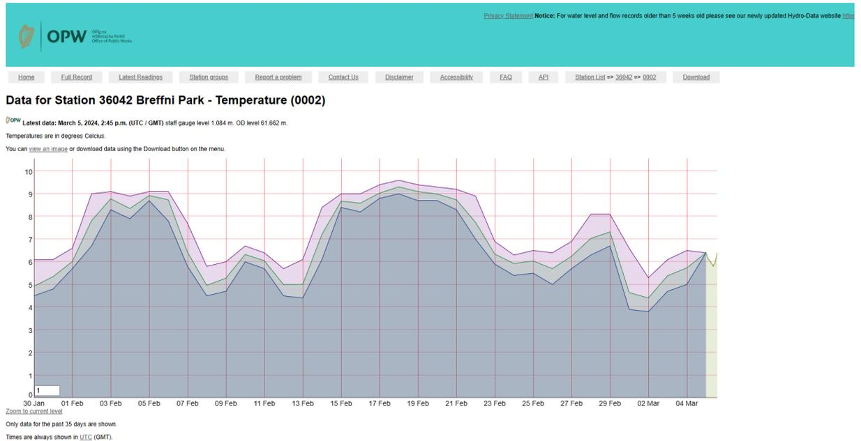
Temporal Temperature profiles indicate winter temperature variations in the order of 3.5°C, with river temperatures fluctuating between around 6°C and 9.3°C.
