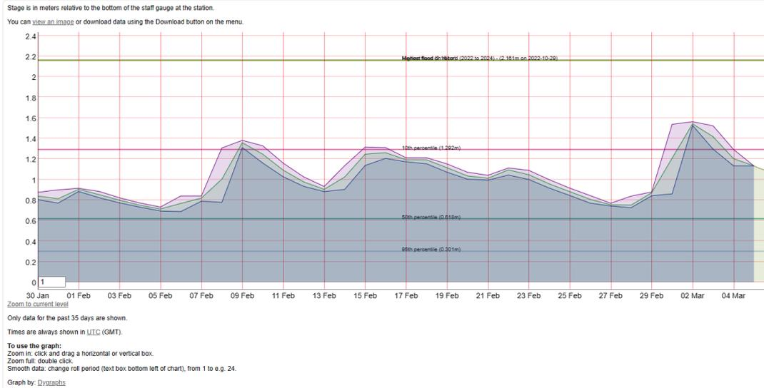
OPW record a river base level of 60.578mOD for this location and the data indicates winter water levels fluctuating by around 1m in this stretch of the Cavan River.
